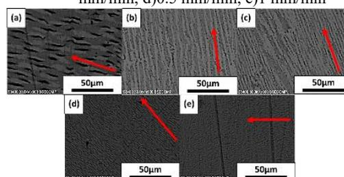
Fig. 4. BEI of CsI/CsCl/NaCl eutectic on the vertical cross-section. The growth rate: a)0.01 mm/min, b)0.1 mm/min, c)0.2 mm/min, d)0.5 mm/min, e)1 mm/min. The red arrow indicate pulling direction.
