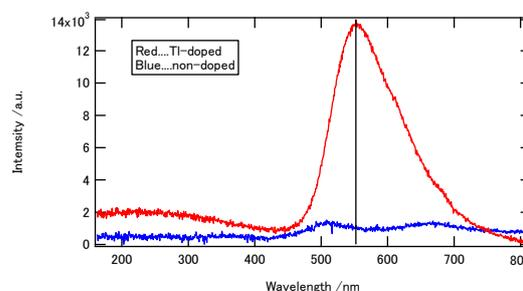
Fig. 5. Radioluminescence spectrum measured under x-ray excitation
