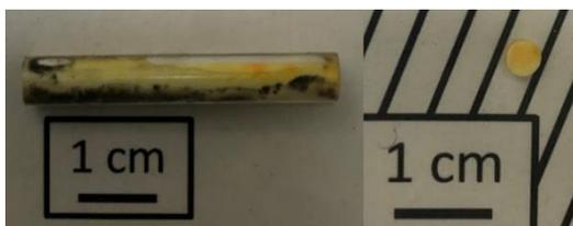
Fig. 2 Example photographs of the grown eutectic as grown. (left) and polished wafer (right).
