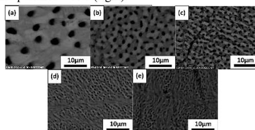
Fig. 3. BEI of CsI/CsCl/NaCl eutectic on the transverse cross-section. The growth rate: a)0.01 mm/min, b)0.1 mm/min, c)0.2 mm/min, d)0.5 mm/min, e)1 mm/min
