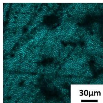
Fig. 6. Image of the luminescence of CsI fibers
