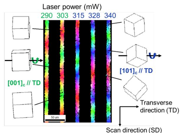
Fig. 1 EBSD orientation map showing the ultralong single-grain crystals obtained on the thermally deposited Al film. A positive pitch rotation of crystal orientation is observed for all the grains. The rotation axis changes from [001]//TD to [101]//TD as the laser power is increased.
