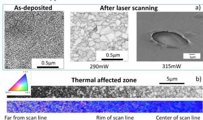
Fig. 2 Solid-state recrystallization of the Au films after laser annealing. a) mean crystal grain size increased ten folds at laser power 290 mW, but ablation occurred at laser power 315 mW. b) The thermal affected zone with extensive crystal growth at the center of the laser scan line.
