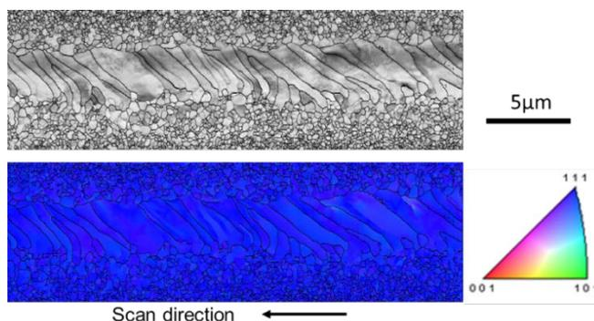
Fig. 3 EBSD image quality map and crystal orientation map of the 50 nm Au film capped with 200 nm SiO<sub>2</sub> after laser annealing. A melting pool was formed at the center, where lateral coarse grains crystallized with a strong (111) crystal texture.
