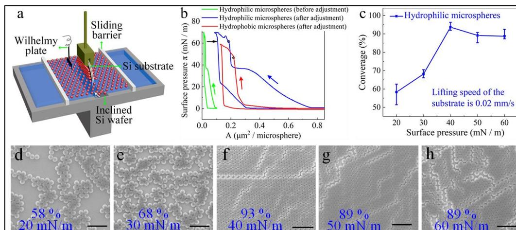
Fig. 1. (a) Schematic illustration of the fabrication process of 2D colloidal crystals using LB method. (b)  $\pi$ -A curves of the 2 types of PS microspheres. (c) The coverage of 2D colloidal crystals on the Si substrate prepared at different surface pressures using hydrophilic PS microspheres. (d-h) SEM figures of the 2D colloidal crystals of hydrophilic microspheres, with surface pressure of 20, 30, 40, 50, and 60 mN/m, respectively. Scale bars in the images are 2  $\mu\text{m}$ .
