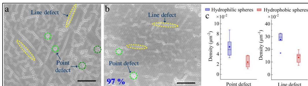
Fig. 3. SEM figures of the prepared 2D colloidal crystals with defects. (a) Hydrophilic microsphere crystal. Point defects include vacancies (light circle) and overlapping spheres (dark circle). (b) Hydrophobic microsphere crystal. (c) Statistics of the defects of the 2 types of colloidal crystals. Scale bars are 5  $\mu\text{m}$ .
