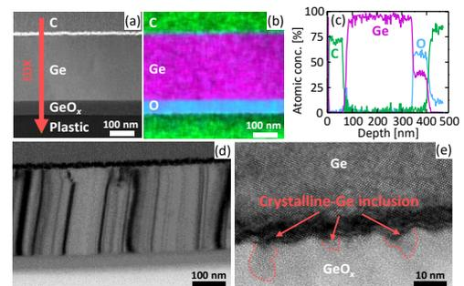
Fig.4 Characterization of the cross-section of the sample for Ge layer grown on plastic substrate after PA. (a) HAADF-STEM image. (b) EDX elemental mapping. (c) EDX depth profile along the arrowed line in (a). (d) Bright-field TEM image. (e) High-resolution lattice images showing the Ge/GeO<sub>x</sub> interface.
