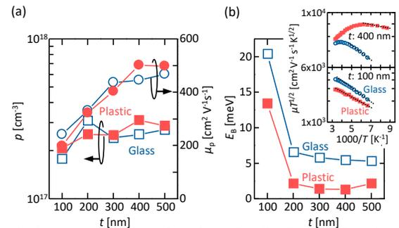
Fig.3 (a)  $p$  and  $\mu$  as a function of  $t$ . (b)  $E_B$  as a function of  $t$ . Inset shows representative Arrhenius plots of  $\mu T^{1/2}$  for  $t = 100$  nm and 400 nm.
