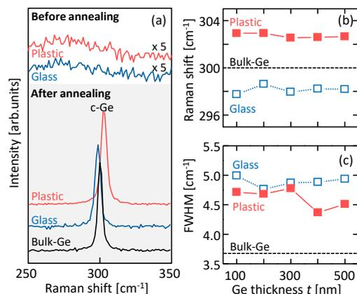
Fig.2 (a) Raman spectra of the samples before and after annealing. (b) Peak shifts from Ge substrate and (c) FWHMs of the Ge-Ge peaks as a function of  $t$ .
