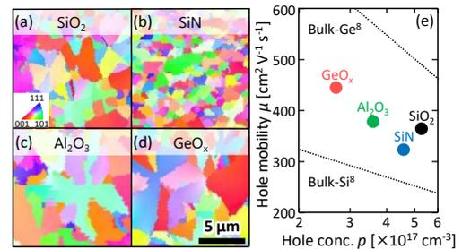
Fig.1 (a)-(d) EBSD images of the 300 nm thick Ge layers with various underlayers. (e) Underlayer dependence of electrical properties.
