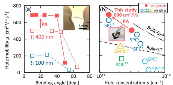
Fig.5 (a)  $\mu$  as a function of bend angle for  $t = 100$  nm and 400 nm. (b) Comparison of  $\mu$  and  $p$  of Ge films on insulators.
