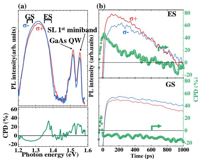
Fig. 2 (a) Circularly polarized time-integrated PL spectra and corresponding CPD at 2 mW for undoped sample. (b) Circularly polarized PL time profiles and corresponding CPD for ground state (GS) and excited state (ES) of QDs at 2 mW.
