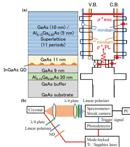
Fig. 1 (a) Schematic of sample structure and PL measurement principle in this study. Capping layer was undoped or p-doped. (b) Schematic of circularly polarized time-resolved PL system.
