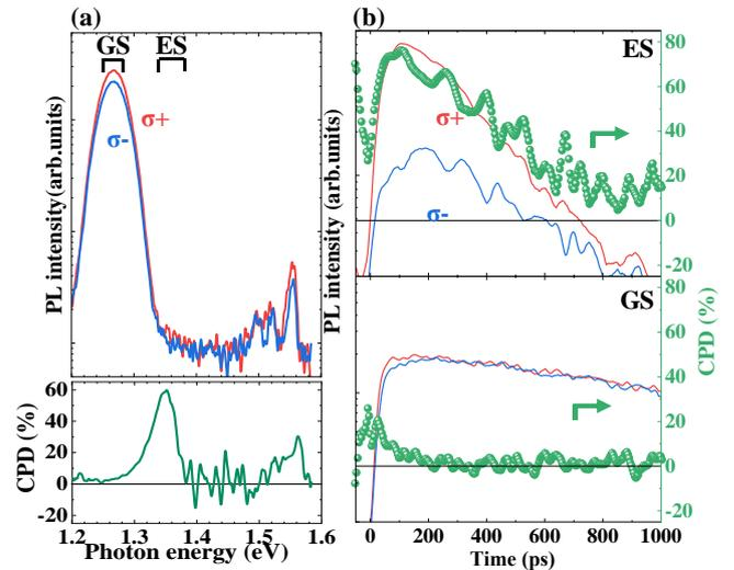
Fig. 3 (a) Circularly polarized time-integrated PL spectra and corresponding CPD at 2 mW for p-doped sample. (b) Circularly polarized PL time profiles and corresponding CPD for ground state (GS) and excited state (ES) of QDs at 2 mW.
