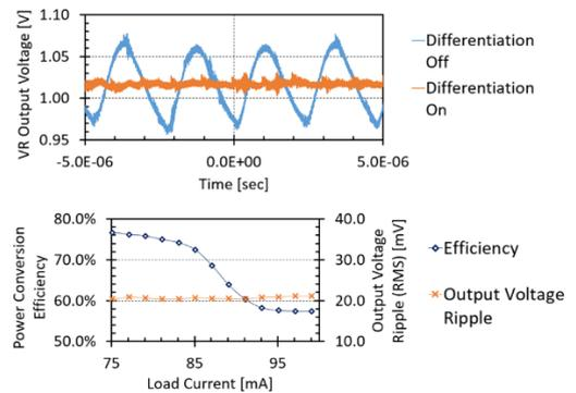
Fig. 6: Upper: Time Domain Waveform of VR Output Voltage with Comparator Differentiation Term On / Off, under Load Current = 250 mA (Measured), Lower: Evaluation of Seamless Transition between LDO and SCVR Modes (Measured)
