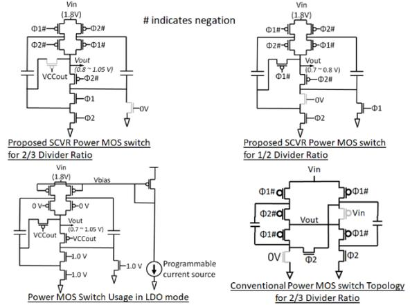
Fig. 4: Power MOS Switch Topology (Proposed vs. Conventional)
