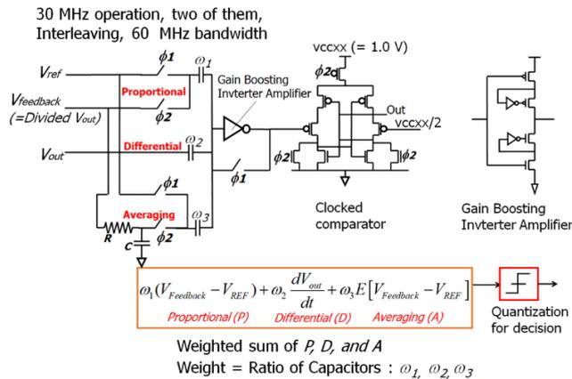
Fig. 2: Proposed Switched Capacitor (SC) Proportional-Differential-and-Averaging (PDA) Comparator Circuit Implementation
