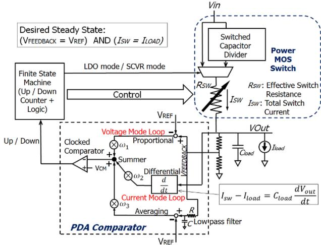
Fig. 1: Functional Block Diagram of Proposed Hybrid Digital LDO / Switched Capacitor Voltage Regulator
