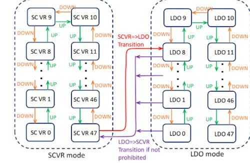
Fig. 3: Finite State Diagram of Proposed Hybrid Digital LDO / SC VR Digital Feedback Controller
