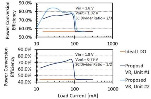
Fig. 5: Power Conversion Efficiency of Proposed Hybrid Digital LDO / SCVR Regulator (Measured)
