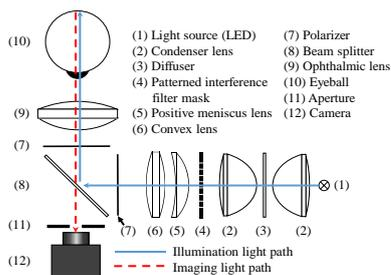
Fig. 4 Schematic diagram of our proposed fundus camera system.
