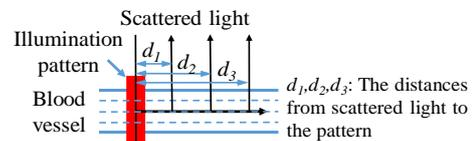
Fig. 3 Schematic diagram of scattered light.
