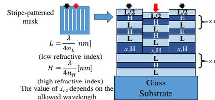
Fig. 2 Schematic structure of the patterned interference filter.
