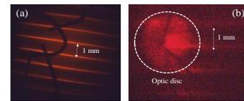
Fig. 6 Stripe patterns (a) in the glass eye model, and (b) in human eye fundus. The pitch and line widths on the mask are 1 mm and 50  $\mu$ m, respectively.
