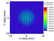
Fig. 5 Simulated illumination pattern on the retina. The widths of the lines of the illumination filter and the spaces between them are both 250  $\mu$ m.
